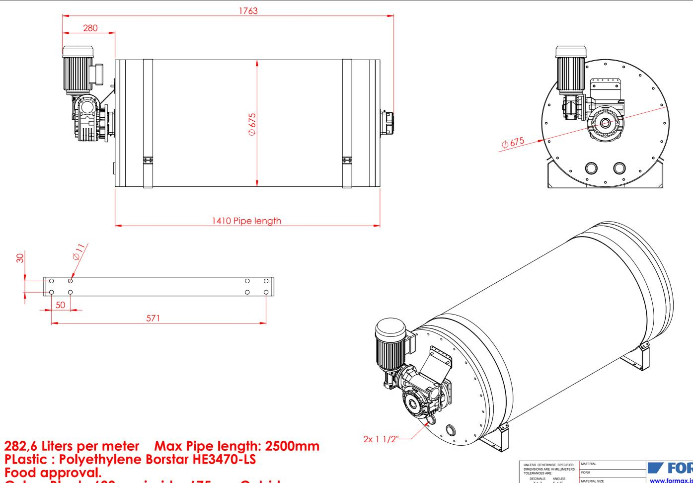
Color: Black 600mm inside 675mm Outside Agitator: °sn/min 7 Motor 0,37kw 3x400V 50/60hz
